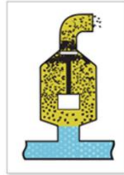
Negative flow rubbish 'bird nest' caught in valve. Blocked and/or leaking.
