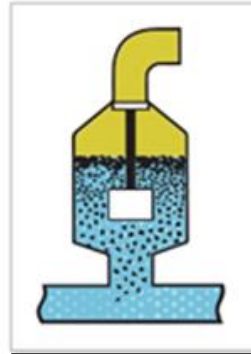
Fats and rubbish accumulate at high point.
