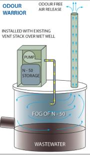
This Odour Warrior can take the place of large or small carbon filters, odour beds and other odour control measures at a fraction of the cost and minimal space requirements.
